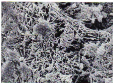
Scanning electron micrograph of a flake of rusty bodywork from a Ford Cortina car, showing a crystalline area of rust.
