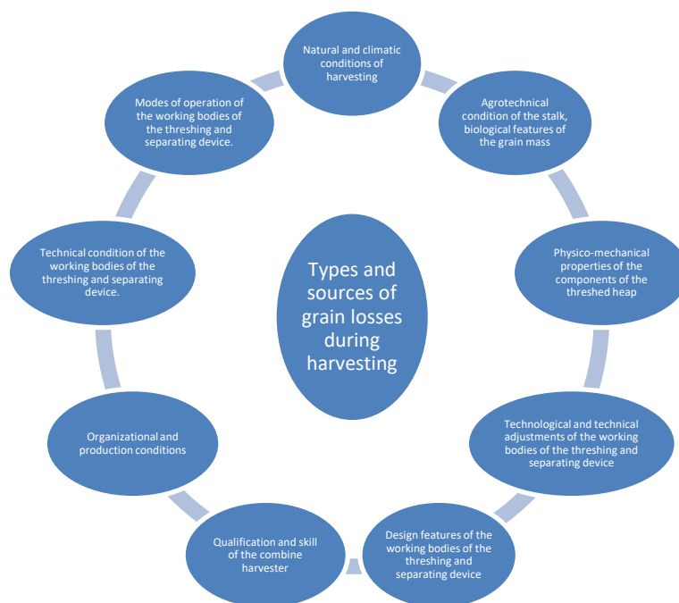
Fig. 1. Causes and factors determining the amount of losses and mechanical damage to grain during harvesting
