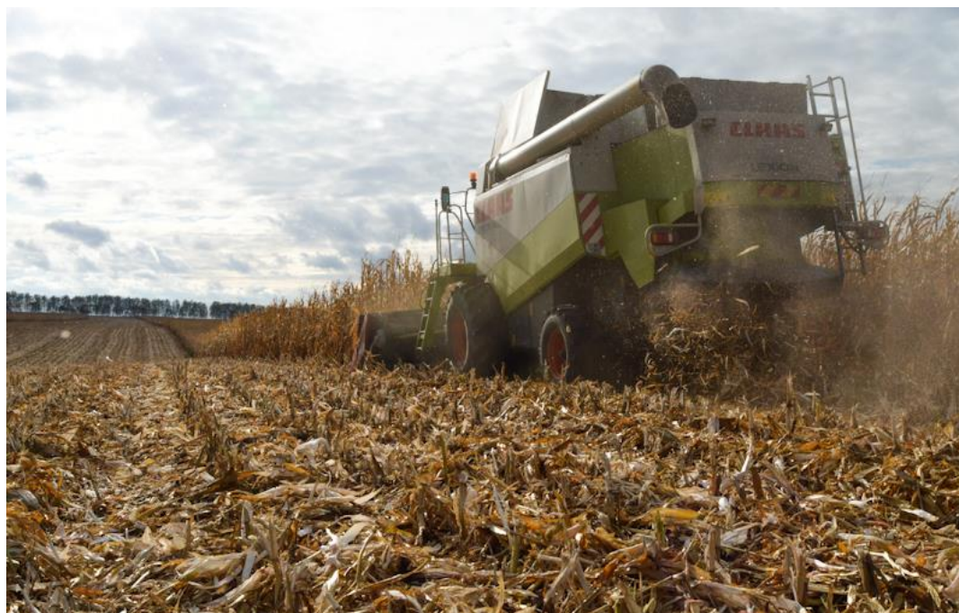
Fig. 1. Grain-harvesting combine with a multi-drum threshing and separating device
