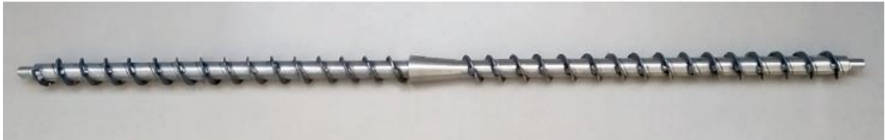
Fig. 1. The screw of an electromechanical hydrolyser
