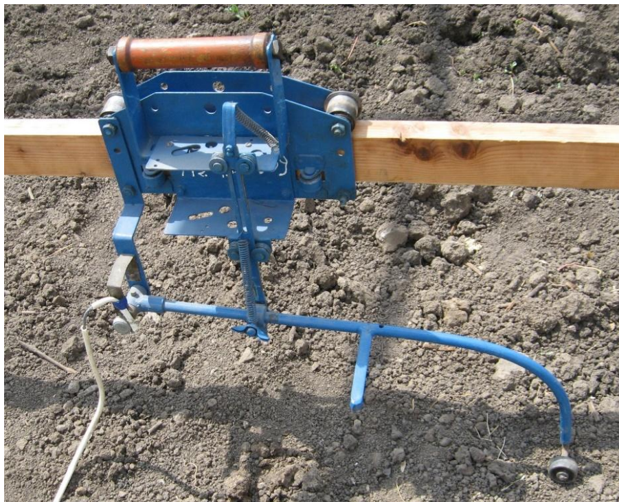
Fig. 2. Device for recording fluctuations of the profile of the field surface
