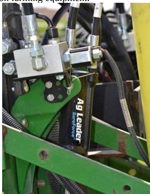
Fig. 7. Sure Force hydraulic clamping system from Ag leader
