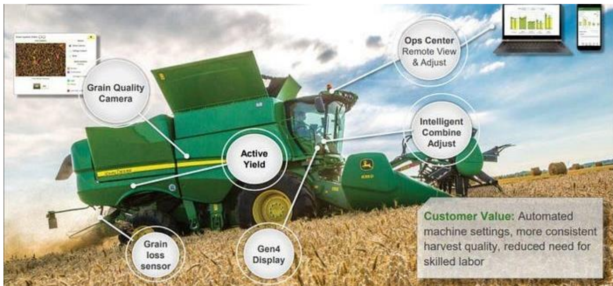
Fig. 2. The parts of a combine harvester.
