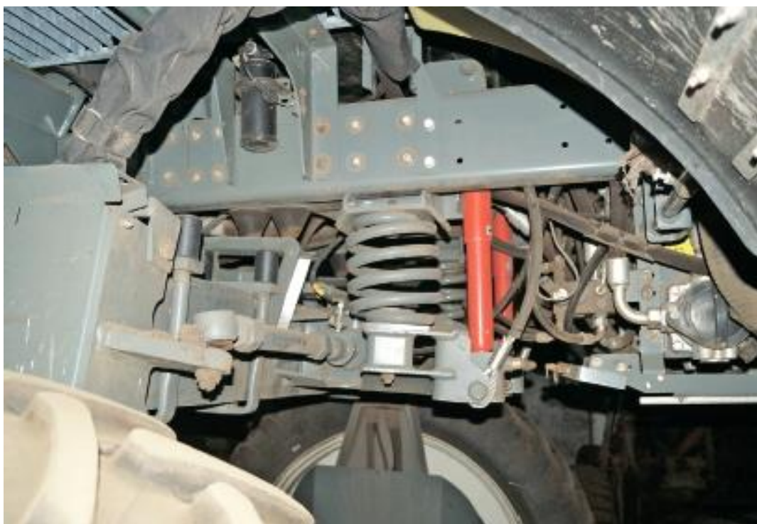
Fig. 4. Technical condition of mechanical suspension of self-propelled sprayer.
