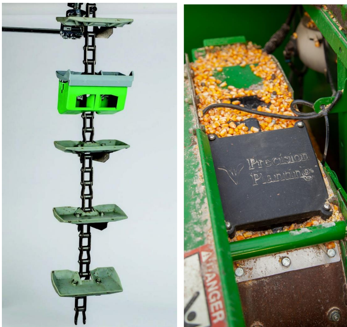
Fig. 1. Grain elevator and the yield sensor installed on the combine.
