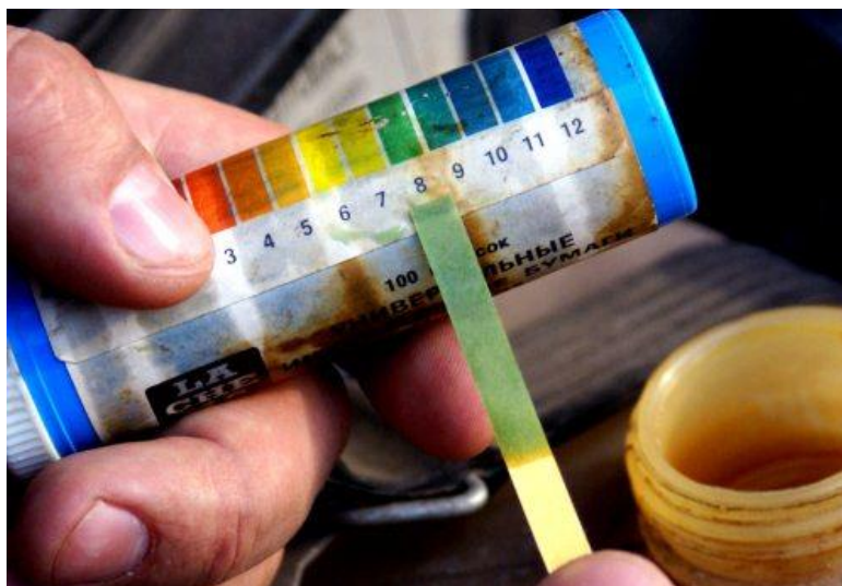
Fig. 1. – The pH measurement of the coolant by means of indicator paper (pH 8)
