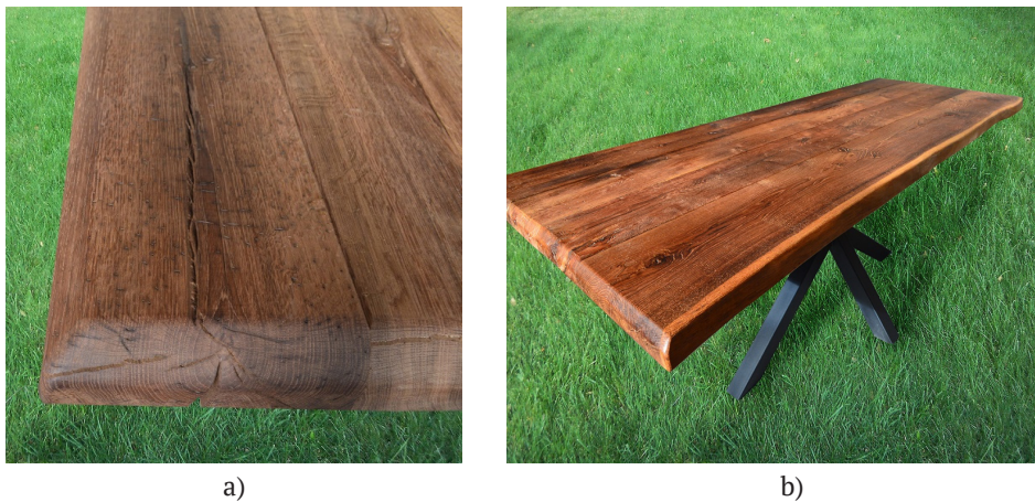
Figure 7. Table made of thermally modified oak wood: a – part of the tabletop that shows the passages of insects; b – general view of the table
