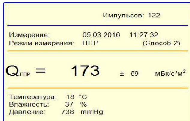
Fig. 3. Values of the meter when measuring RFD in soil on Vynnychenko Str.
