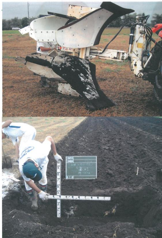
Fig. 77. Deep ploughing with tractor-driven reversible mouldboard plough (Japan, 2011).
