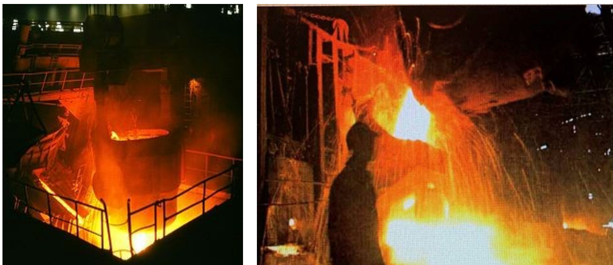
Fig. 2. Cast iron pouring into an open-hearth furnaces
