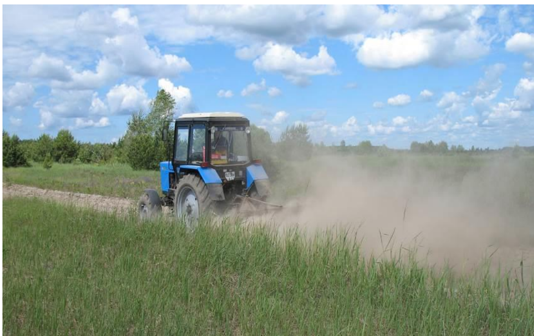
Figure 9. Establishment of fire breaks generates radioactive dust that can lead to an increase of inhalation doses for tractor drivers. Photo: V. Yoschenko.
