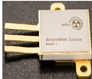
Figure 1. General view of the BetaVolt power supply
