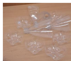
Fig.2. Parts of a PET bottle to obtain a ribbon by cutting and shredding into flex; a-lid; b-bottle blank without a bottom; c-separated parts of the bottom and neck
