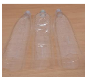
Fig.2. Parts of a PET bottle to obtain a ribbon by cutting and shredding into flex; a-lid; b-bottle blank without a bottom; c-separated parts of the bottom and neck
