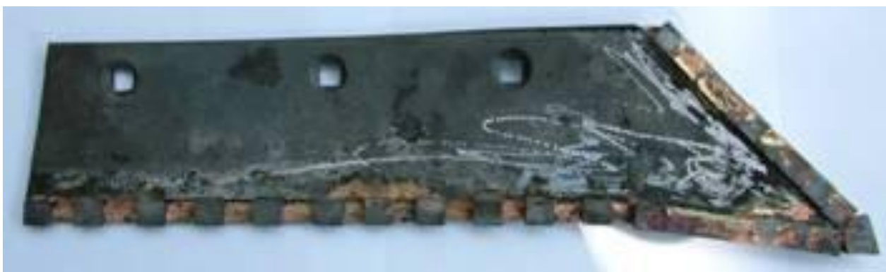
Fig. 2. Ploughshare, soldered to the front of the metal-ceramic plates with their solid position.
