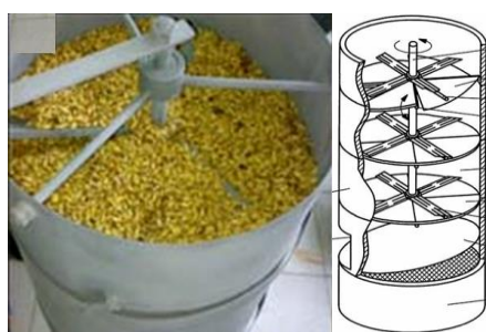
Fig. 4. Dryer with mixing of the material layer
