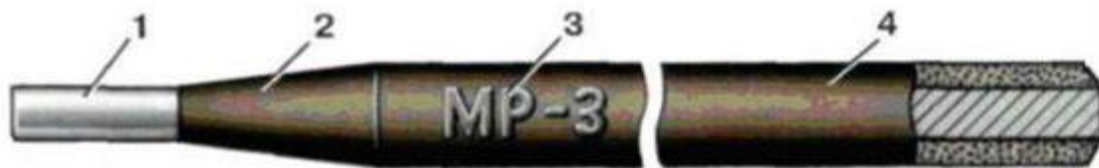
Fig. 3. The structure of the welding electrode: 1 - rod, 2 - transition section, 3 - electrode mark, 4 - coating.
