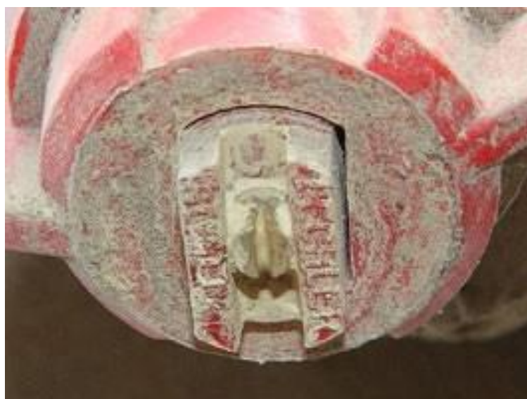
Fig. 1. Coked sprayer - the sprayer was not washed after treating with fungicide.
