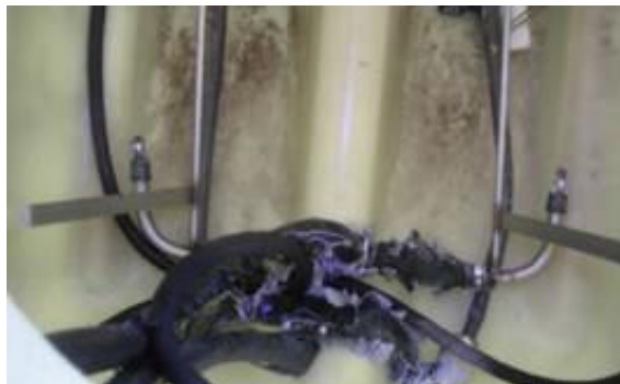
Fig. 2. Tubes and hoses after testing cheap generics
