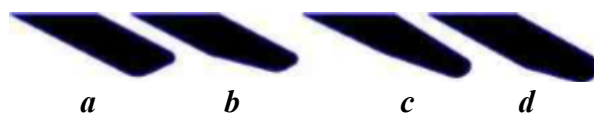
Figure 4 - Changes in the profile of the cutting elements of the tines on different soils: a and b - loamy; c and d - clay (40 and 80 hectares of operation)
