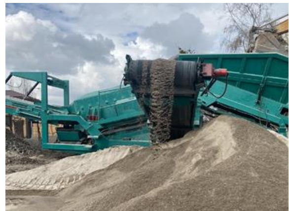
Figure 3 – Powerscreen Warrior 1400 tracked screening plant in operation during the pilot project conducted by Neo-Eco in Hostomel
