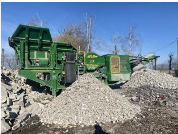
Figure 2 – McCloskey J40 jaw crusher in operation during the pilot project implemented by Neo-Eco in Hostomel
