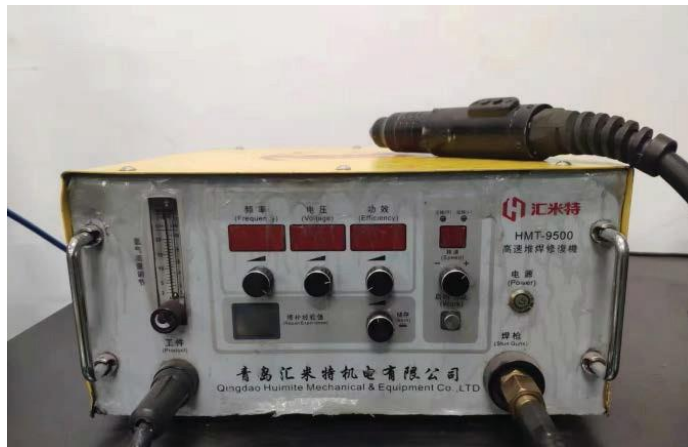
Fig. 1. The high-speed ESD repair machine (HMT9500)
