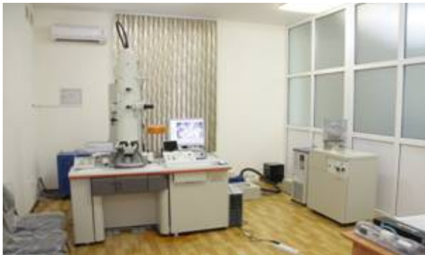
Transmission electron microscope JEM-1011, complete with a CCD - digital camera Morada (OLYMPUS)
