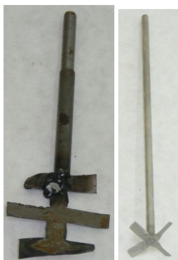
a) b) Fig. 1. Stirrers: a – bladed with three blades on the shaft; b - four-bladed with inclined blades.
