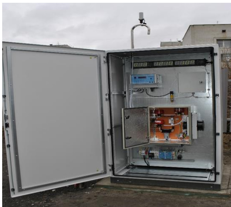
Figure 6.13 – Stationary post of the automated atmospheric air monitoring system of the Kiev Regional State Administration
