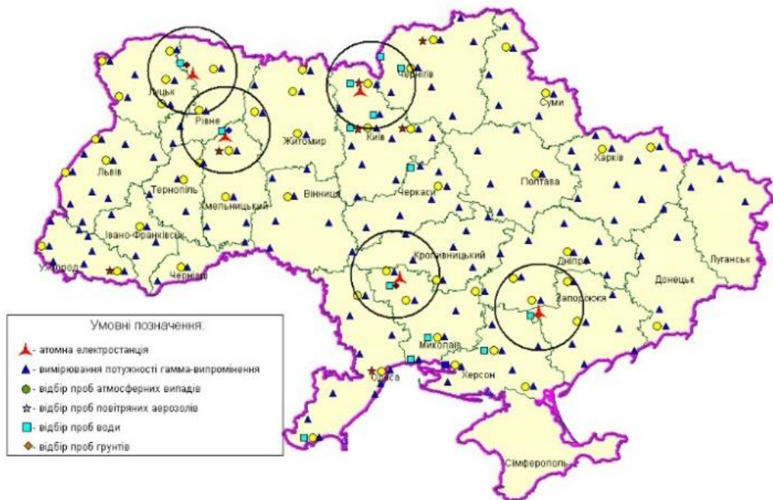
Figure 10.16 Map-scheme of location of hydrometeorological service observation points for radioactive contamination of the natural environment on the territory of Ukraine
