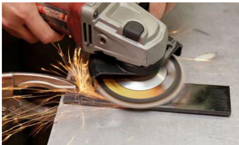
Figure 1 – a' Stripping of metal by portable electric grinder
