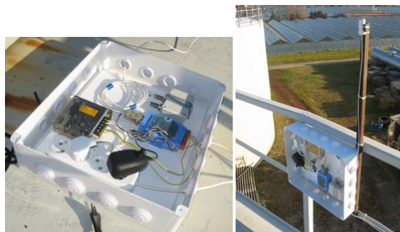
Fig. 5.1 Information Measurement System of solar radiation intensity
