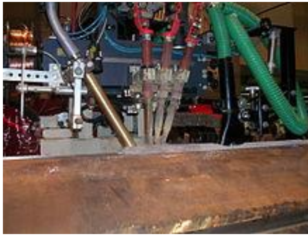
Fig. 1. Submerged arc welding
